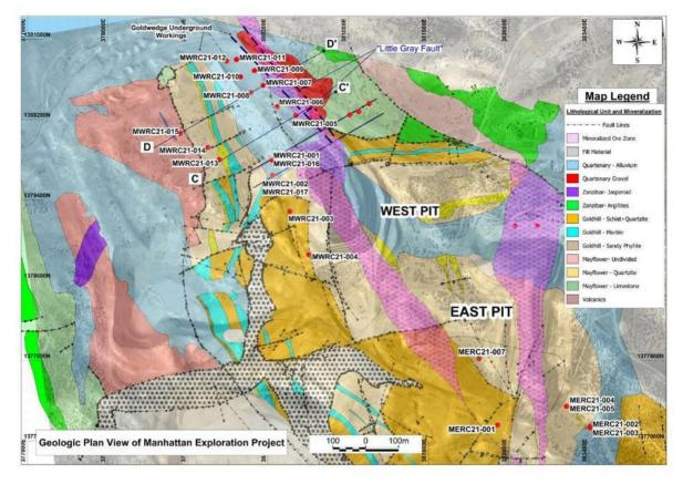
**Figure 1.** Geological map of the Manhattan Mine area with red circles showing drill collar locations and hole IDs indicating holes completed to date. C-C' and D-D' mark cross sections presented in Figures 2 and 3.
