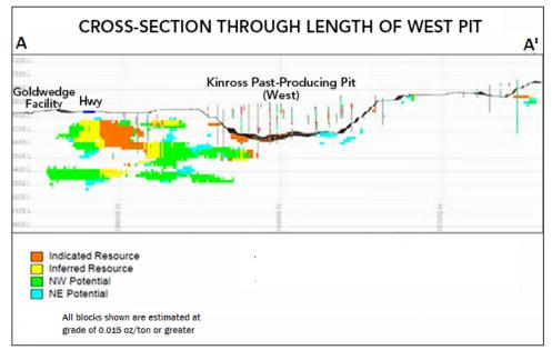
**Figure 3:** Cross-section A - A' showing indicated, inferred resources and potential (Re: Manhattan Divestment Proposal document – Kinross Gold Corp. October 21, 2016). The resource calculations are internal and have not been verified by an independent qualified person according to NI 43-101 guidelines.
