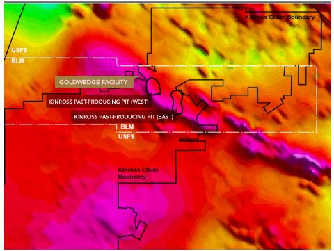
**Figure 4:** Airborne magnetic survey data (Re: Manhattan Divestment Proposal document – Kinross Gold Corp. October 21, 2016). The magnetic anomalies display the probable structural trends of the mineralized sheared metamorphosed interbedded limestones, argillites and phyllites of late Cambrian age.
